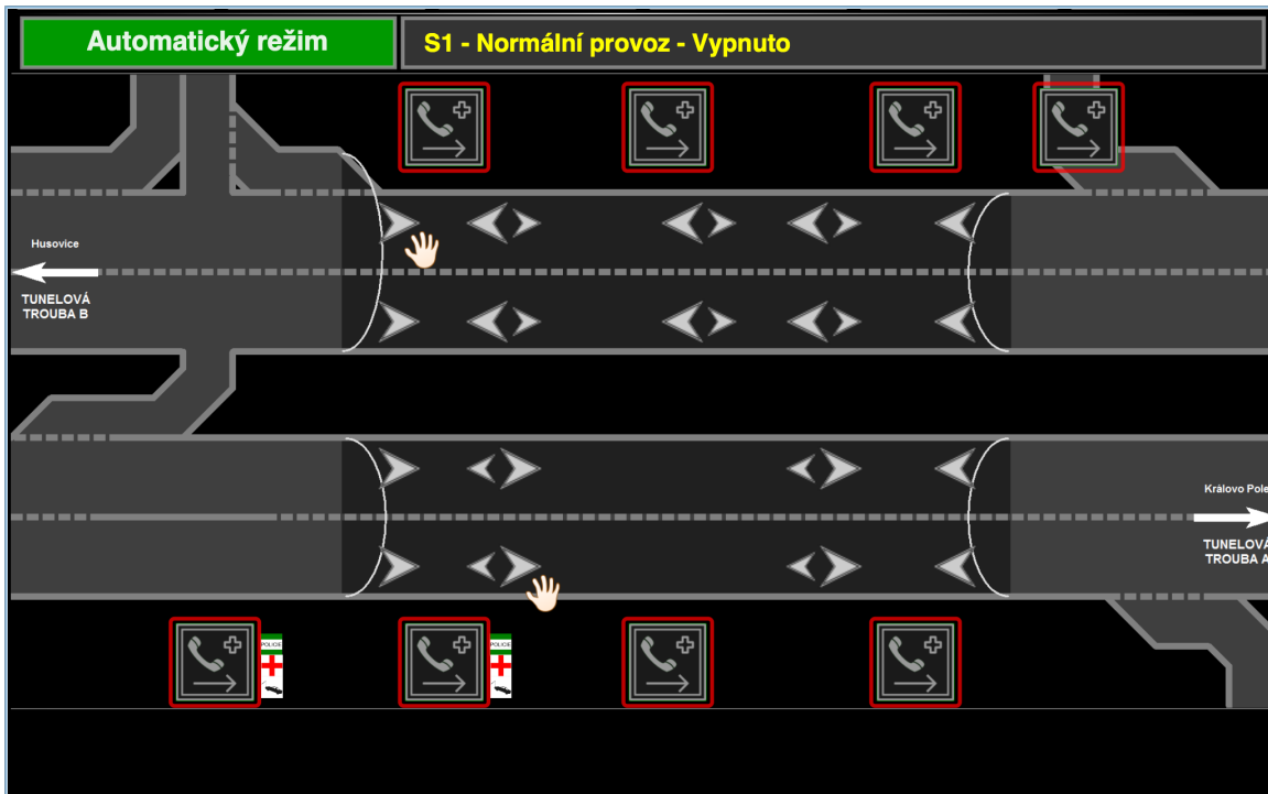
Status of Emergency Phones (SOS Call Boxes) in the tunnel.
