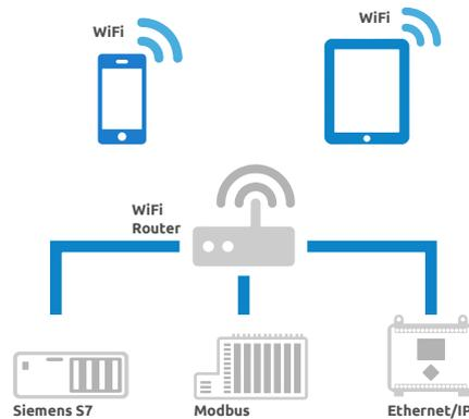
The most important for the future is definitely the first one – OPC UA (Unified Architecture). It is maintained by the independent organisation to ensure better connectivity with the PLCs and RTUs. Surely, most PLC manufacturers will provide OPC UA native driver for their PLCs in the near future.
